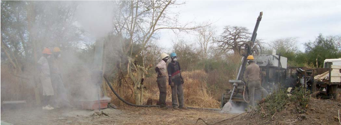
Fig. 1 Rotary Air Blast Drilling Source: Analyst
